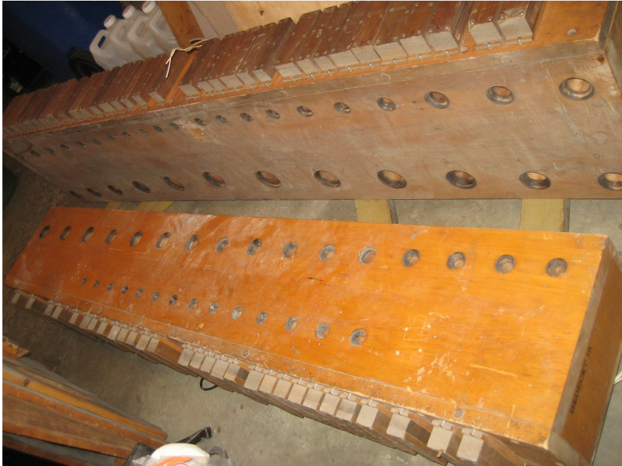
32 note electro-pneumatic Casavant Bourdon chest 30 note electro-pneumatic Casavant Gedekt chest
